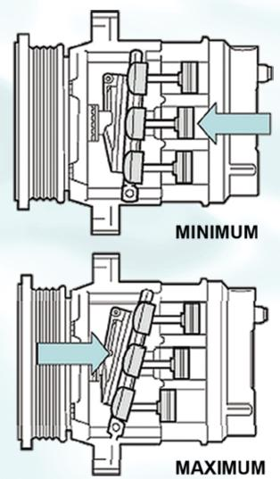
The swash plate in a variable displacement compressor is "hinged" so it can tilt at different angles. The higher tilt creates greater piston movement and higher pumping volume, or displacement, of refrigerant. When the swash plate angle is almost perpendicular to the compressor shaft, it generates almost no refrigerant displacement and consumes negligible energy.
