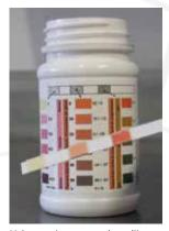
Using coolant test strips will tell you the condition of the antifreeze/water mixture.
