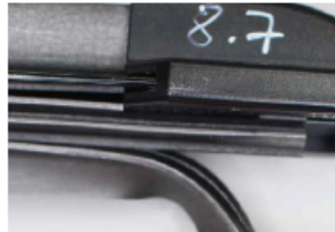
Valeo HydroConnect: Cracked wiper blade lip
