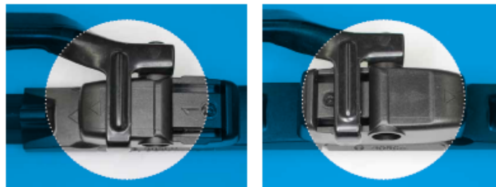
It is possible to install the Bosch AP24U adapter the wrong way round (left: correct fitting, right: incorrect fitting)
