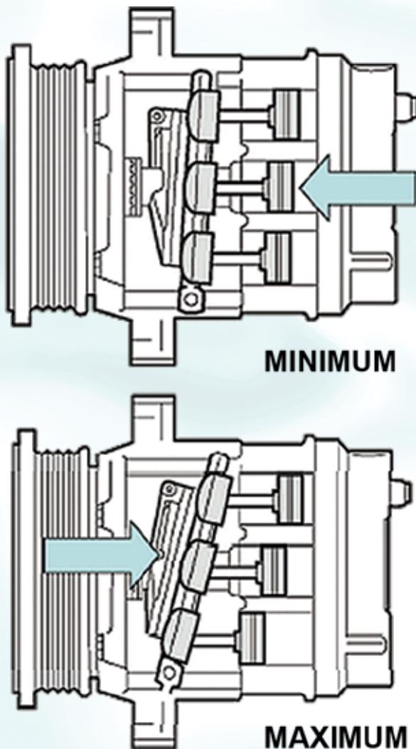
The swash plate in a variable displacement compressor is “hinged” so it can tilt at different angles. The higher tilt creates greater piston movement and higher pumping volume, or displacement, of refrigerant. When the swash plate angle is almost perpendicular to the compressor shaft, it generates almost no refrigerant displacement and consumes negligible energy.
