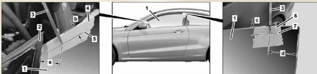
To adjust the height, start by making reference marks on some tape placed near the top edge of the glass as shown. See the text for the dimensions.
