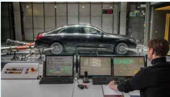
Testing a new Mercedes-Benz equipped with a CO<sub>2</sub>-charged AC system
